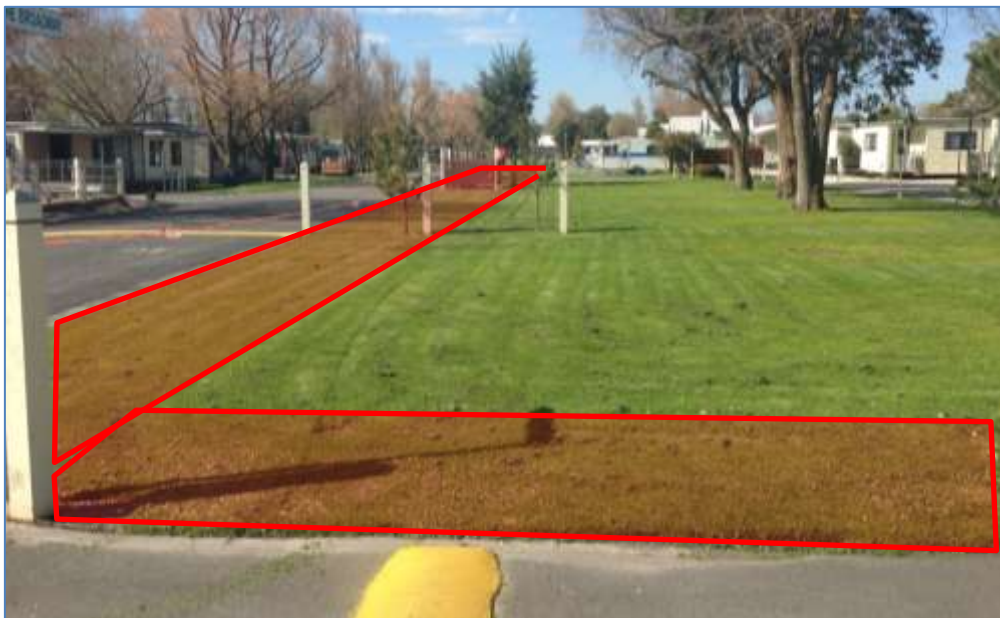
Figure 5.5: Illustration of setback envelope to be kept clear of vehicles and objects that will obstruct sight distances
