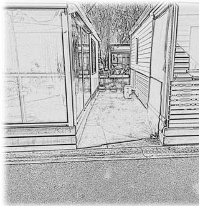
Figure 4.4: Showing restricted visibility due to lack of setback from road
